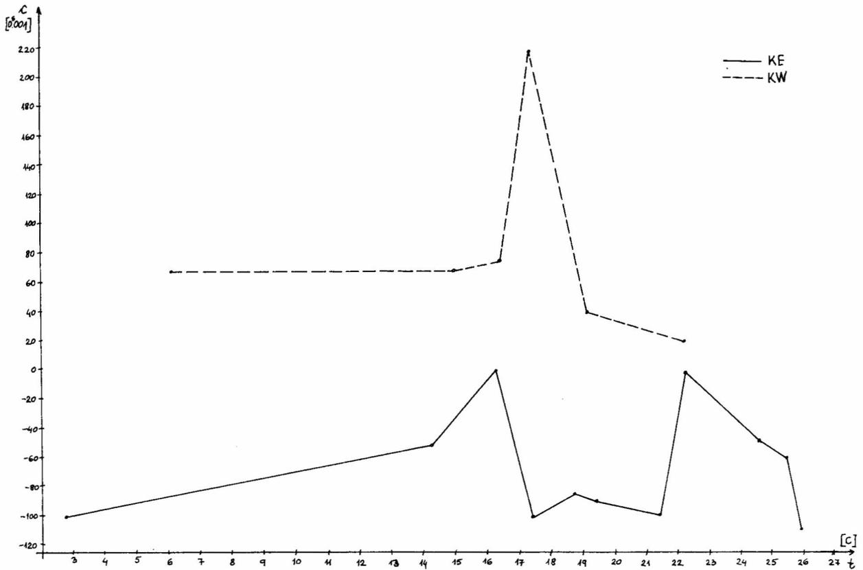
Fig. 1. Collimation  $c$  dependence on temperature during observation
