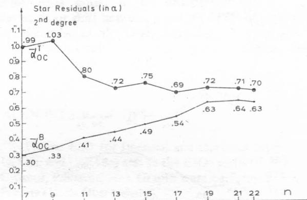
Fig. 3. Precision on Reductions in  $\alpha$  by the 2<sup>nd</sup> degree bijection. Bijection between sky and plate:  $X = a_{00} + a_{10}x + a_{01}y + a_{20}x^2 + a_{11}xy + a_{02}y^2$ ,  $y = b_{00} + b_{10}x + b_{01}y + b_{20}x^2 + b_{11}xy + b_{02}y^2$ .
